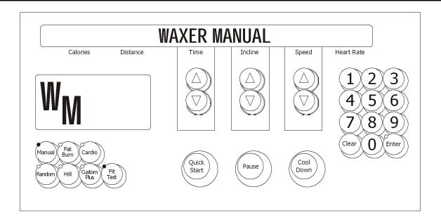
Upon entry into this test the letters WM (waxer manual) will be in the profile window. This test allows the user to manually fire the waxer system. It allows the user to see information concerning the waxer motor as well. The waxer information will scroll automatically every 3 seconds.
